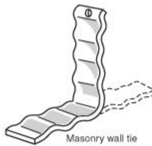
FIGURE 12.6.2.1(c) Masonry Clearance Reduction System.
